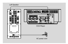
After everything is connected properly, plug in the AC power cord to the power socket.
